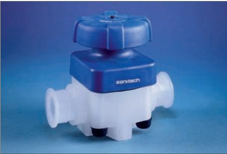
For use in high-purity water, chemical and process lines. Valves have a smooth fluid path with no pockets to harbor bacteria or contaminants. Fluid comes in contact with only two valve components, the body and diaphragm. These valves can be pneumatically actuated.
