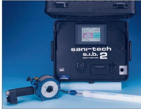
The Sani-Tech® S.I.B.® 2 fusion welding tool is a better way to install high-purity plastic piping systems. S.I.B.® technology creates a smooth interior surface at the tubing weld, eliminating all beads, crevices, and intrusions into the fluid stream. The smooth surface reduces the areas for contaminants and bacteria to collect. The updated S.I.B.® 2 tool delivers faster weld times and increased weld identification and traceability, and also offers improved durability and ease of use.
